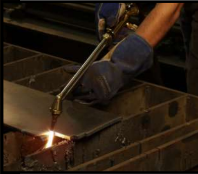
Model MK-300 shown cutting with 75° head
